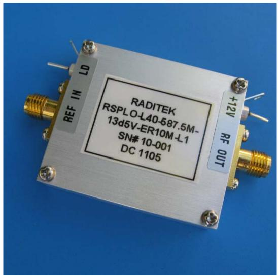
RADITEK's new DRO based, synthesizer product line can be configured as a fixed frequency phase locked DRO, which unlike conventional Phase locked DROs does not require a reference frequency that is a sub multiple of the output frequency. The output frequency can be to over 25GHz. Another option is to have some limited tunability with only a small reduction in Phase noise over a pure fixed DRO type. Reference can be 10MHz, 100MHz etc. Contact sales@raditek.com for more information.
